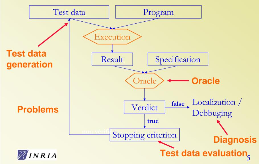
Dynamic transformtation testing process
