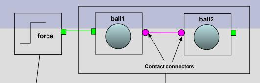
The contact connectors do not necessarily connect state-information (as normal connectors do).
