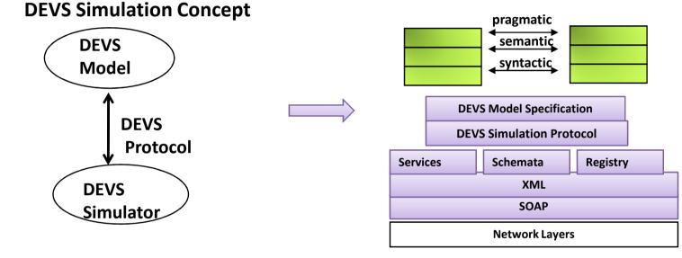
DEVS Protocol specifies the abstract simulation engine that correctly simulates DEVS atomic and coupled models
