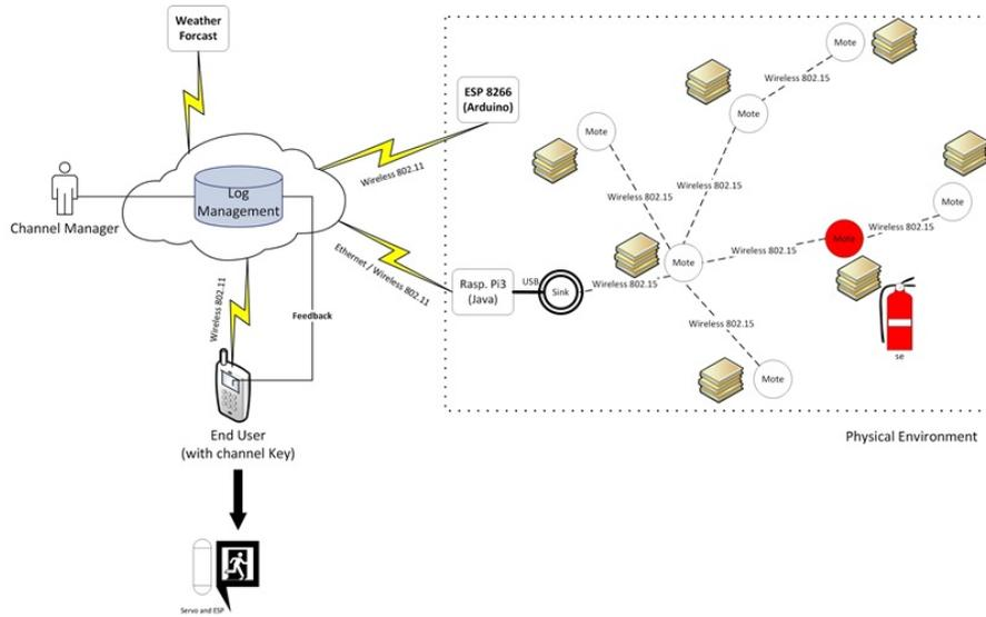
Figure 1: The architecture of fire detection system.
