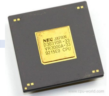
32 bit MIPS R3000 processor (115000 transistors) early 1990s
