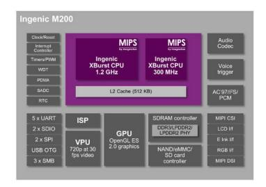
Smart watch SoC has dual MIPS cores
