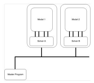
As we can see in the image, all the simulation kernels (model + solver) are connected to a bus. The master program as well is connected to the same bus. Now we create a co-simulation environment where parts of the whole simulation can be swapped with new, better or faster algoritms.
