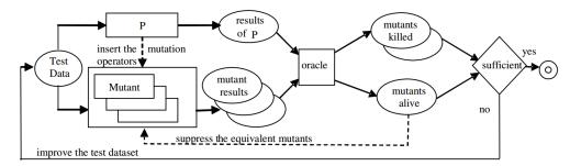
In this graph, courtesy of [2], P is the program to be tested, the testing suite is in the form of the test data (input) and the oracle, which "kills" the detected mutants. Any mutants left over that are not equivalent to P are then used to improve the test dataset.
