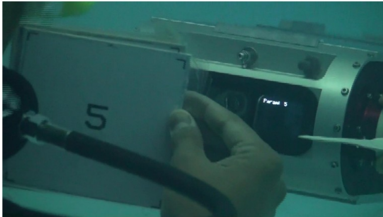
(c) Example of command acknowledgement given on the LED screen of the Aqua2 robot during field trials.
