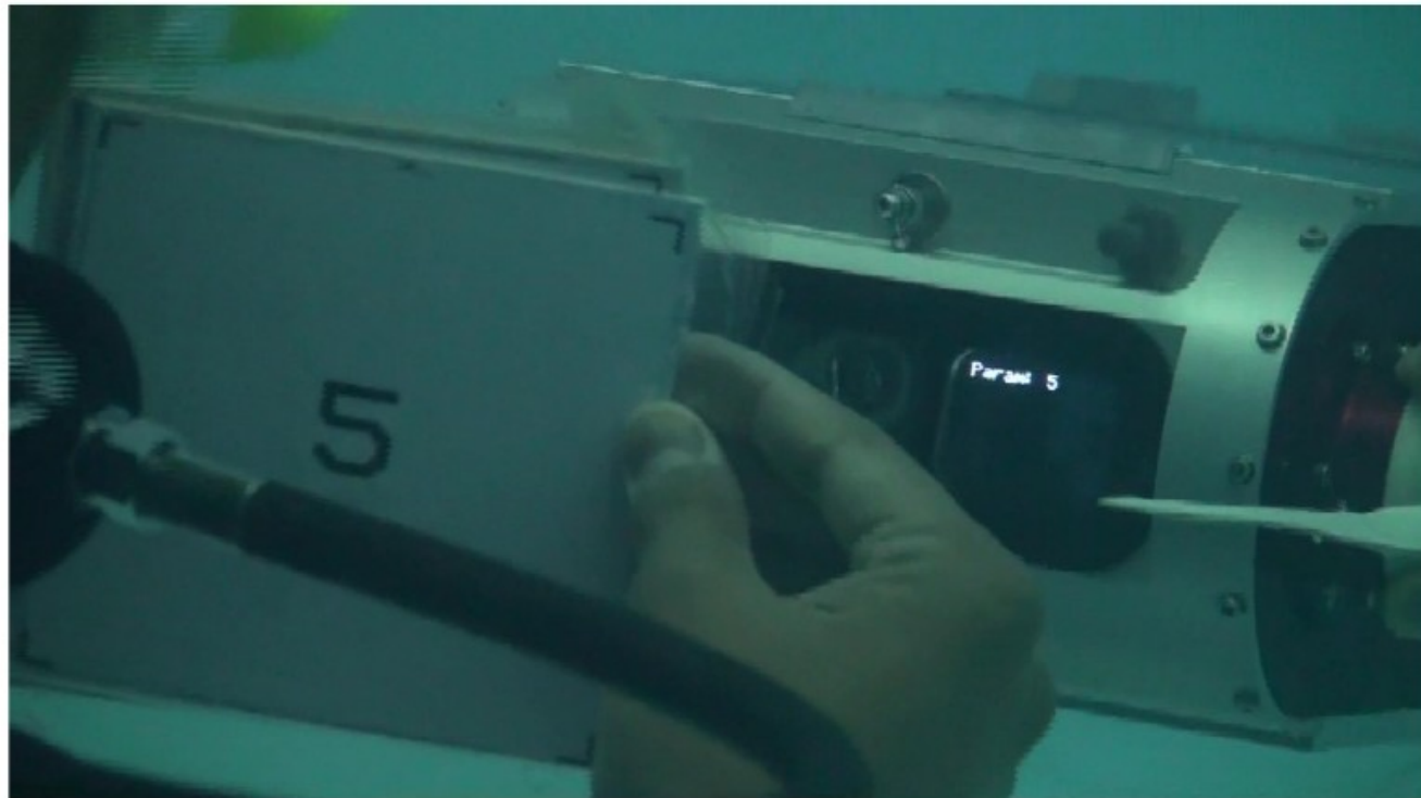
(c) Example of command acknowledgement given on the LED screen of the Aqua2 robot during field trials.
