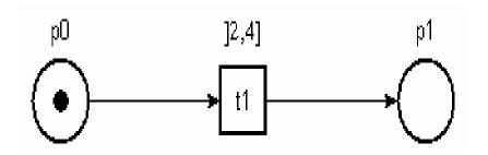
Times a and b for transition t1 are relative to the moment at which transition t1 is enabled.
