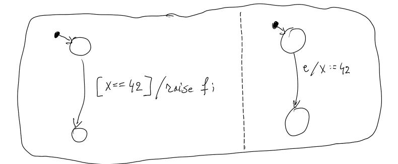
NO, because the guard condition [x==42] is evaluated BEFORE the assignment to x. Not until the next RTC step (caused by ANY input event), will event 'f' be raised. Transitions that have only a guard condition can be a great source of confusion, when the Statechart also contains after-triggers:
