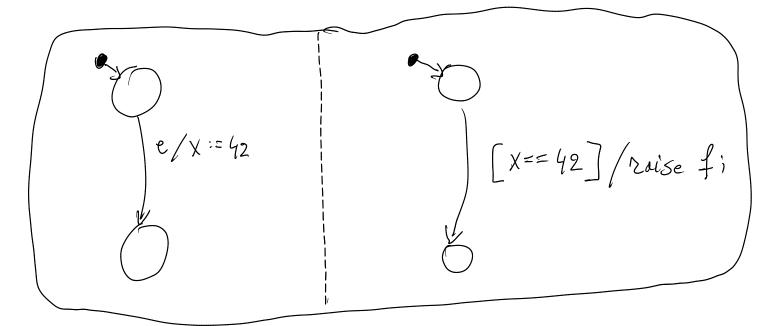
YES, because guard condition [x=42] is evaluated AFTER the assignment to x, but in the same RTC step in which event 'e' is received.
