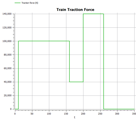
Figure 10: Train traction force F_{traction} profile.
