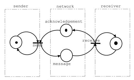
The above Petri Net (Activity Diagram) models a simple communication between a sender and a receiver. It is assumed messages are not lost nor damaged. A token in the sender place means the sender is ready to send. A token in the receiver place means the receiver is ready to receive. A token in the acknowledgement place means there is an acknowledgement (of receipt) message on the network. A token in the message place means there is a data message on the network.
