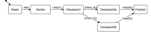
Figure 2.3: Sequence of algorithm steps modeled as a statechart
