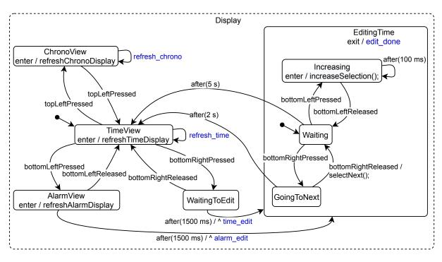
Figure 4.7: Display region of digital watch Internal events are blue.
