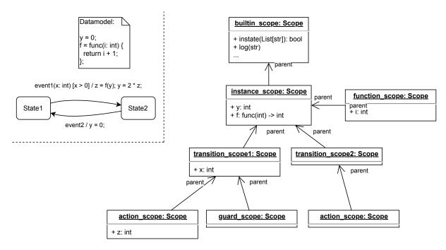
Figure 3.21: A statechart model (upper left) and its hierarchy of scopes
