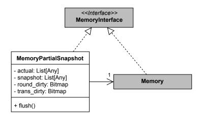
Figure 3.27: Class diagram of MemoryPartialSnapshot class. Dark-gray classes defined in action language package.
