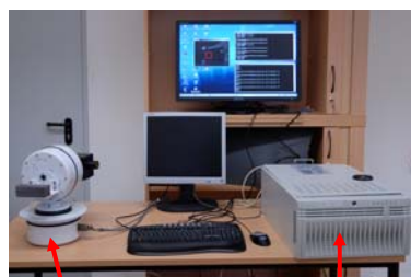
Pan-tilt-unit with mounted camera
