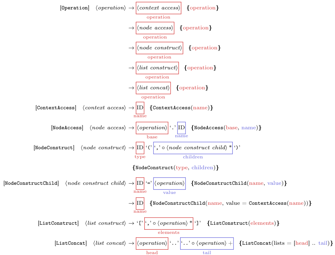
Figure 8.29: Grammar specification for the concrete textual syntax of TCF annotated with TCF models and expected types. The start symbol is \langle operation \rangle .
