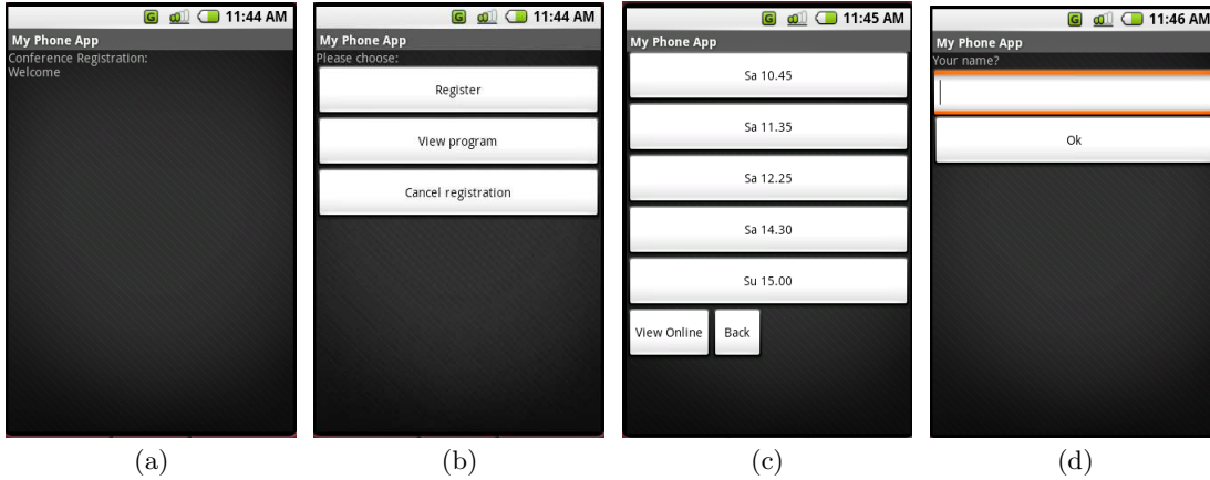
Figure 6: Screenshot of the synthesized application running on a Google Android device emulator: (a) The Welcome screen; (b) The ActionChoice screen; (c) The ProgramSchedule screen; (d) The EnterName screen.
