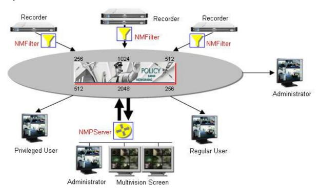
**NMPServer** is installed in the central site. It receives all the requests and dispatches all the requested streams. **NMFilter** is installed on the recorders. The **NMPServer** and **NMFilter** set have to manage 3 different policies:
