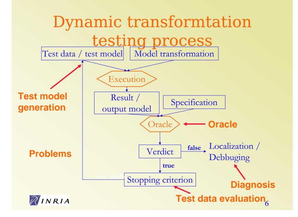
Dynamic transformtation testing process
