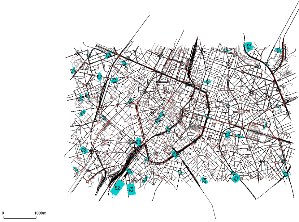
Figure 14: Position of lane area detectors (virtual sensors), colored in green, in a model of the city of Brussels.
